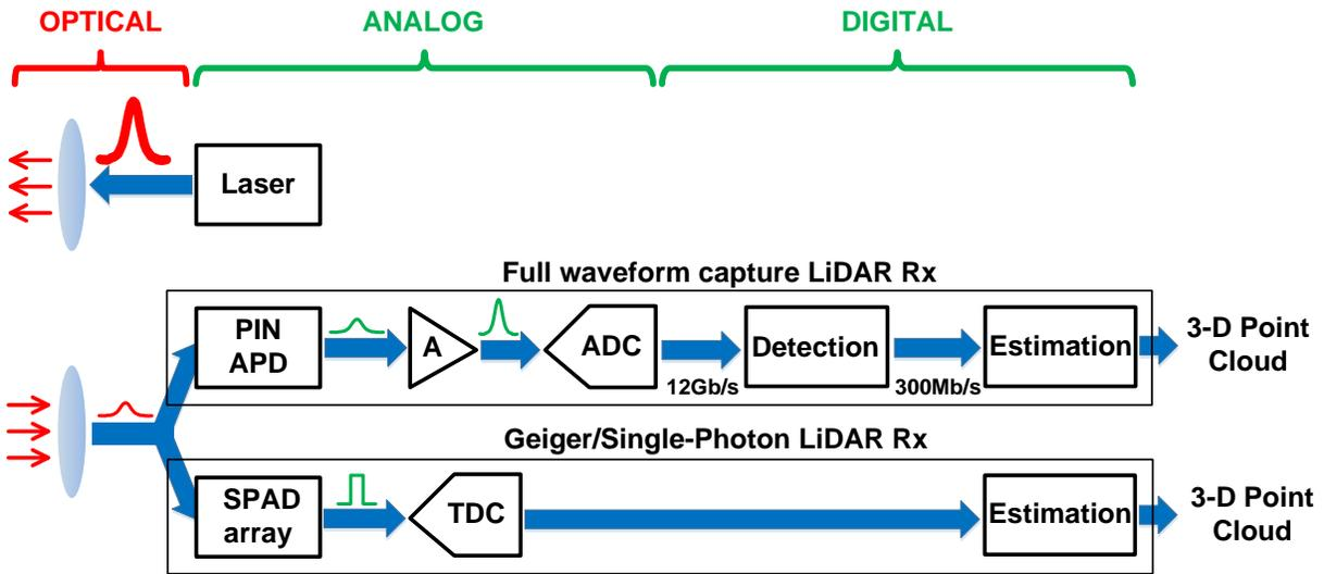
Figure 1. Example of a LiDAR system
